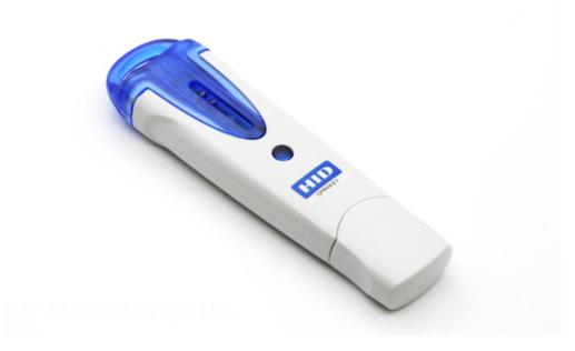
The 6121 USB SIM reader from Omnikey (previously the CardMan CM6121) is a high speed USB 2.0 device encapsulated in a grey and transparent blue case. This reader is fully PC/SC and EMV Level 1 compliant and supports all ISO 7816 SIM-sized smartcards. It also meets USB CCID specifications for simple installation.
